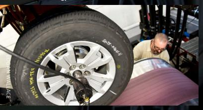
The hub of the National Tire Research Center is an \$11.5 million force-and-moment machine (LTRe) created for passenger-car, light-truck, and motorsport tires. The LTRe is a superior product representing a transformational leap in technology by offering at least twice the capability in major performance areas across current tire test machines.
