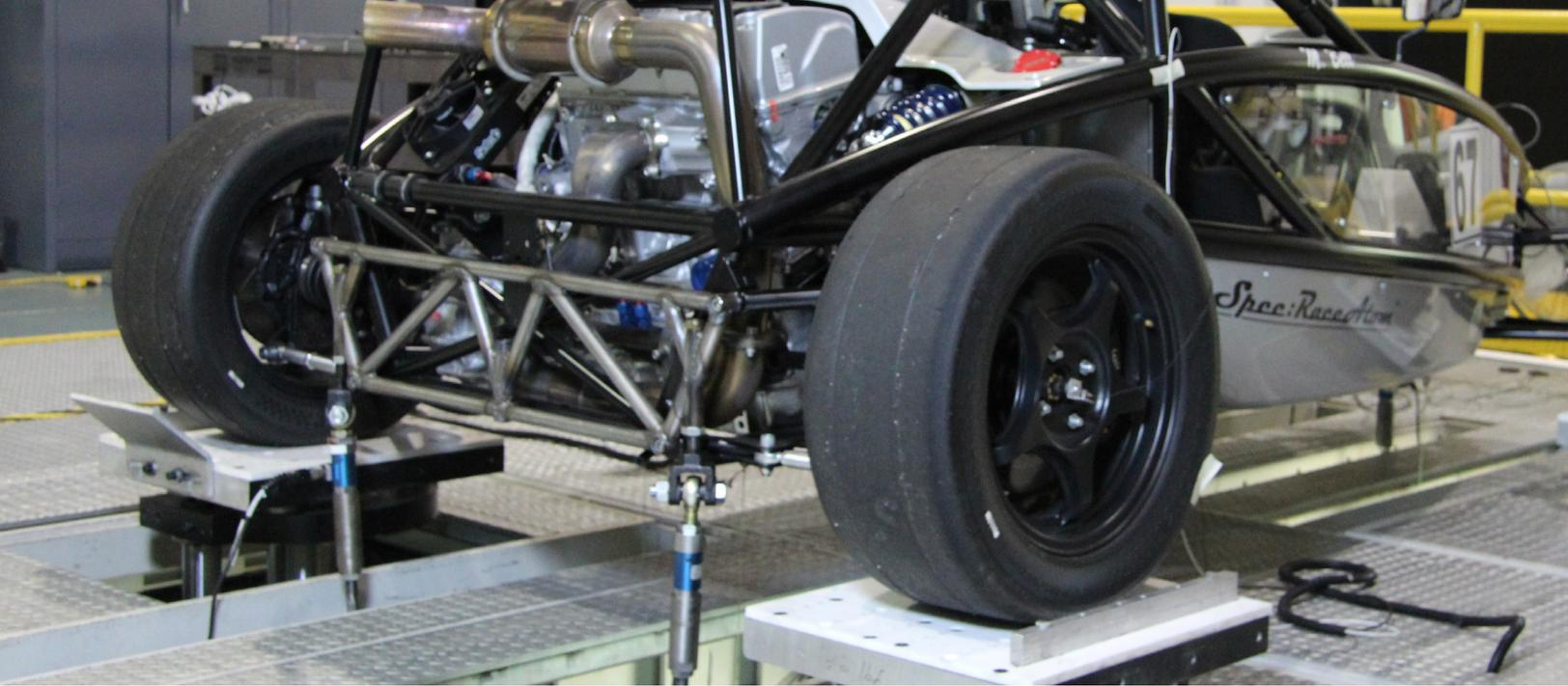
Each of the four wheel platens of the multi-post can produce up to 11,000 pounds (5,000 kg) of dynamic force. Each of the three to four additional downforce actuators can provide up to 4,500 pounds (2,000 kg) of inertial and/or downforce loading. When coupled with 12-inch actuator strokes, the large load capabilities enable a wide variety of road simulations. The wheel platens and downforce actuators are repositionable, allowing for testing of myriad vehicles.
