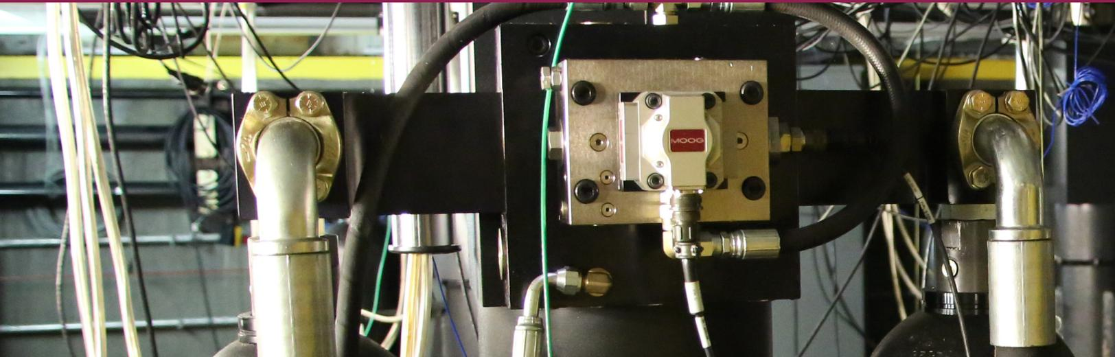
an active aerodynamic downforce application scheme. Through simulation, an aero map can be used to calculate the aerodynamic loads acting on the vehicle, and the resulting downforce loads can be changed dynamically to provide the most realistic lab-to-track tests. The system controller will also allow for other hardware-in-the-loop implementations, such as jacking and dive compensation.
