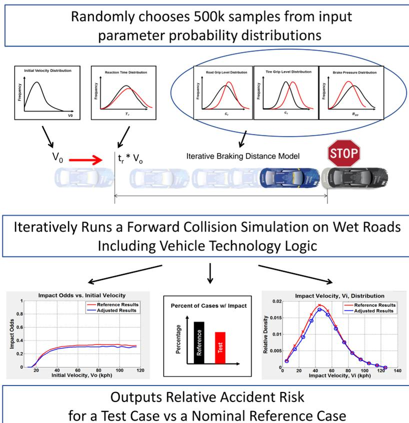
The reference case is based on data available in the market and attempts to represent the US public road situation. A test case can be developed by adjusting any of these distributions to meet a desired study case scenario.
