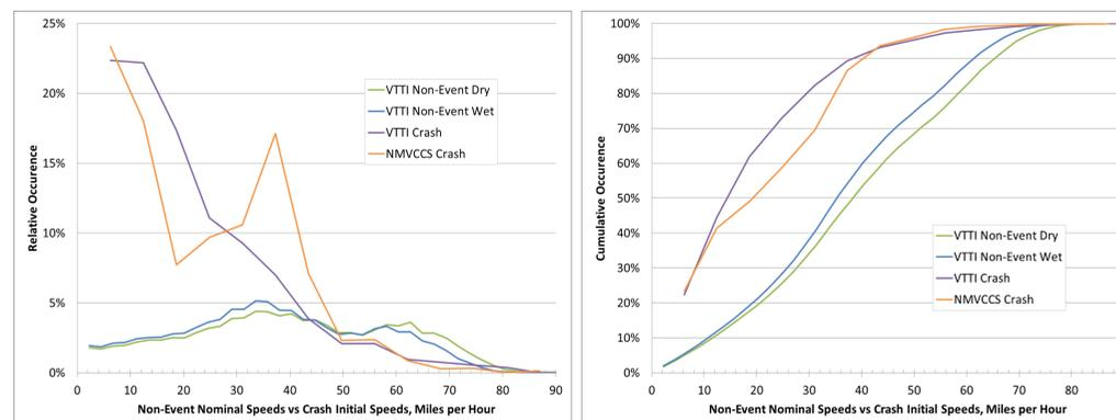
Velocity distributions are compared between wet and dry conditions and between normal "non-event" driving and crash events. This data is then compared to the crash data from NHTSA's NMVCCS database. The model is simulating a wet braking scenario, so the wet non-event speed distribution was used.
