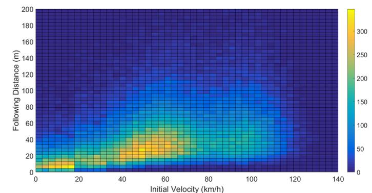
Based on a bivariate distribution for following distance and velocity, a representative distribution of following distances can be found for a selected velocity.
