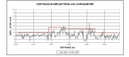
Also delivers characteristic deflection (Dc) in the homogeneous section:  $Dc = Dmax, average + 2.\sigma$
