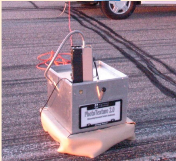
System with fixed four light sources
