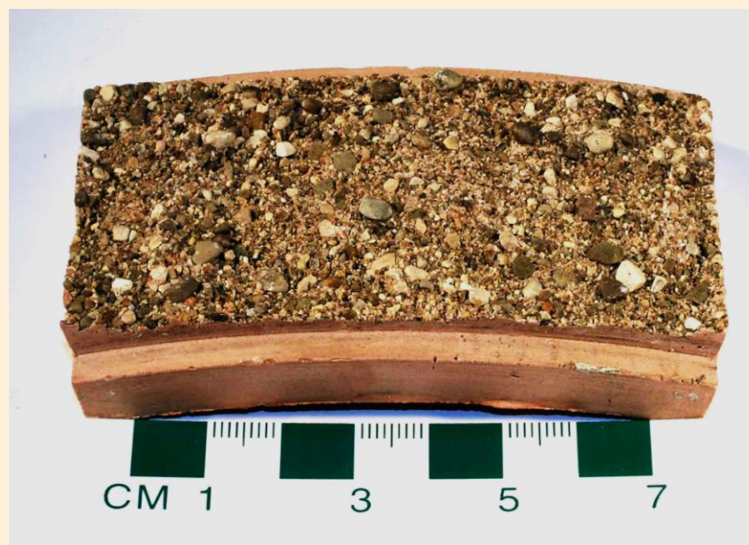
Resin coupons not satisfactory when made with sand
