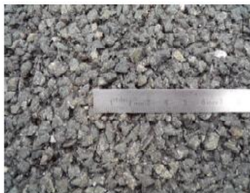
Surface M2: Very thin bituminous concrete (0/6)
