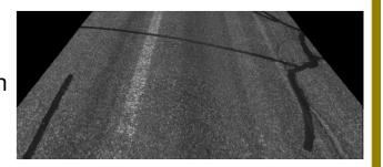
Macro-Texture Measurement using MPD - ASTM E1845-01
