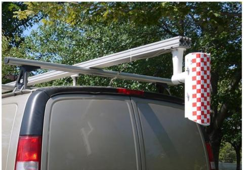
VOTERS has created a color video acquisition and automated analysis system to verify the physical measurements of other sensors in addition to quantification and classification of pavement cracks. Click on any point on the map to see the image of that location and the crack detection results.
