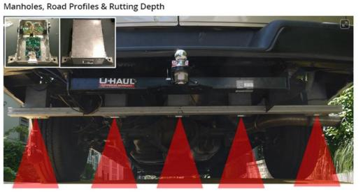
VOTERS millimeter-wave radar systems mounted underneath the van is capable of detecting metal objects on the road and is used to identify the manholes.
