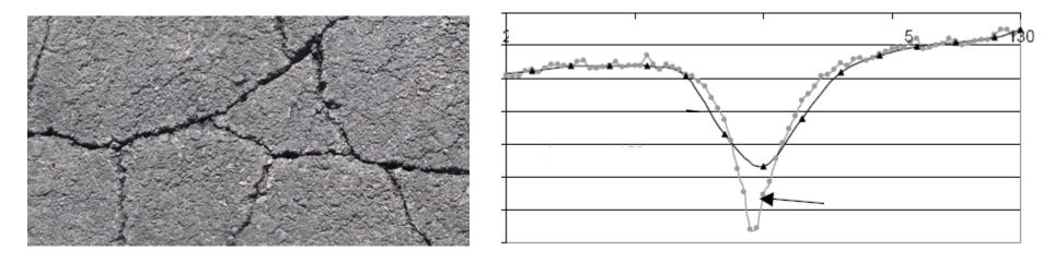
• The problem with laser depth analysis (in addition to cost) is that it will not detect sealed cracks, patches and others.
