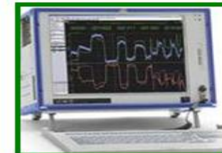
Data Acquisition Unit (16-channel: 2 video, 6 audio, CAN-Bus; all synchronized)
