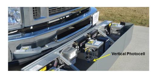
Vertical: Triggers off reflective tape placed on the pavement
