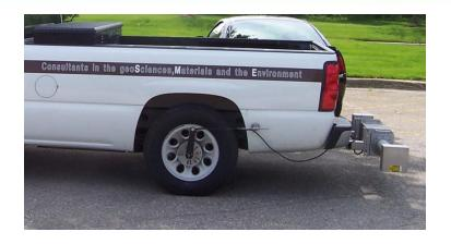
DMI should measure distance with an error of less than 0.15 percent (AASHTO M-328).
