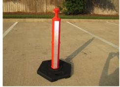
Horizontal: Triggers off reflective mark on a cone placed on the shoulder
