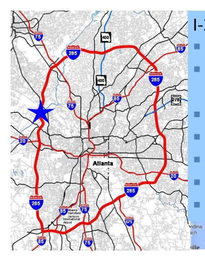
I-285 WB MP 12-13 Constructed in 1968 In service for more than 40 years 10-in thickness No dowel 30-ft joint spacing 12-ft wide Asphalt shoulder
